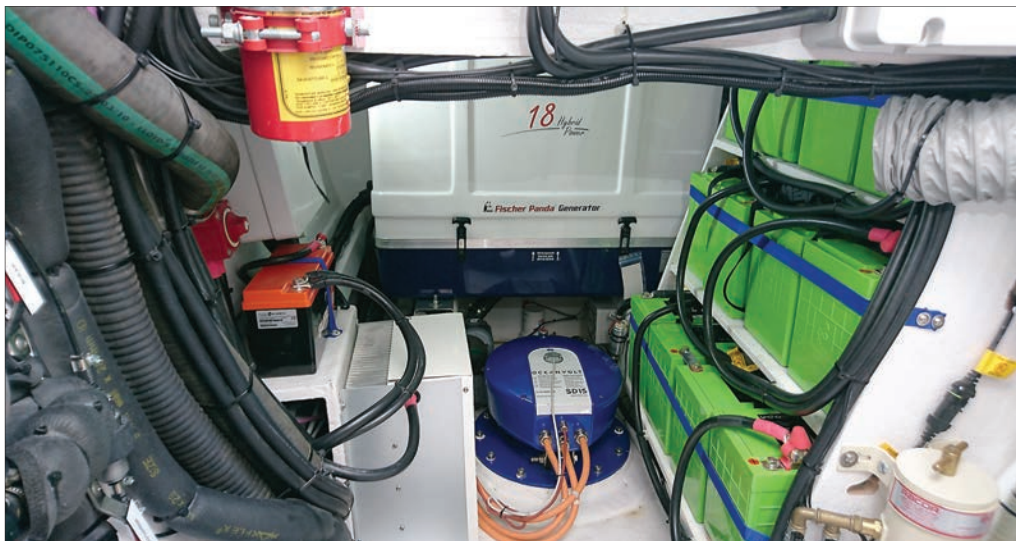
This neat OceanVolt serial hybrid installation includes a large bank of lithium-ion batteries at right and a Fischer-Panda generator in a box at center rear.
