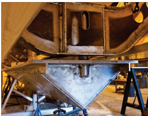
Left —Construction details of the forward sections of America 2.0. Note the marriage of the balsa-cored laminated-cedar hull skin to the aluminum ring frames and keel structure. Right —The welded aluminum lower section of America 2.0's hull and keel sump await attachment to the rest of the wood-and-aluminum hull. Note the massive threaded studs protruding from the flange that will secure the two structures to one another.
