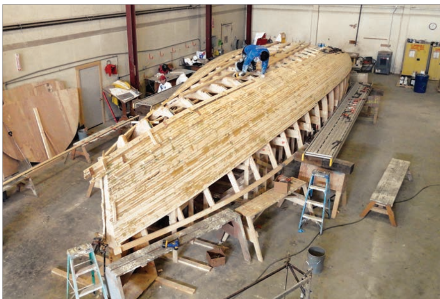
The 47' (14m) excursion daysailer Eleanor under construction in cedar-strip planks at the Scarano shop in 2015. John Scarano characterizes her as a giant vintage International 14.
