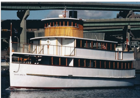
The 65’ (20m) Dutch Apple II was the company’s first experience with an excursion boat. Built in 1989 of laminated wood, the project spurred John and Rick Scarano to move to a larger shop to accommodate the hull and superstructure.
