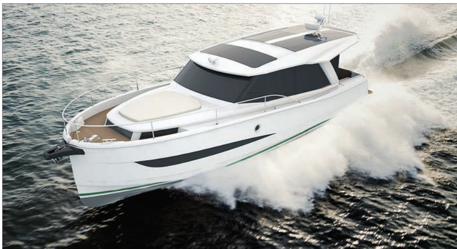
The Greenline 36 (10.9m), the latest in the Greenline family of parallel hybrid cruisers, relies on an integrated flywheel electric machine built into a Volvo Penta D3, and a simple manual selector for electric or diesel propulsion.
