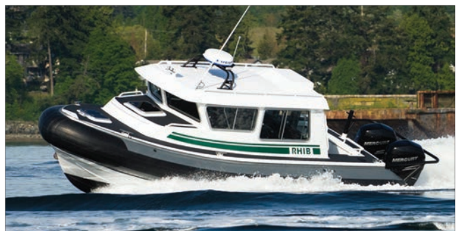
A 30' (9.1m) RHIB in the Knight series can be configured for various applications, including search and rescue. The forward-raked windshield is the preferred style in the Pacific Northwest.
