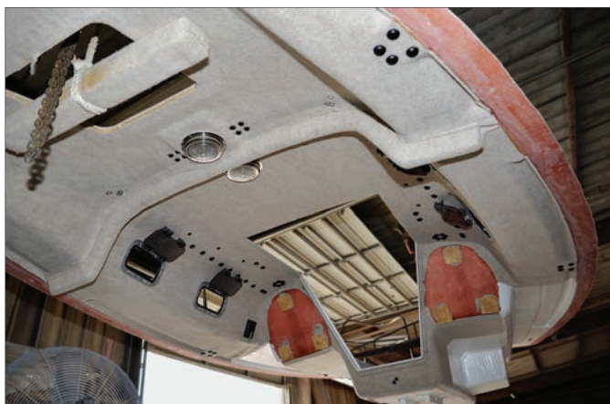
Above —A prewired deck is suspended by overhead chain hoists before it is lowered onto the hull. Right —A shop crew member with a buffing wheel details a hull before moving the boat outside and onto a trailer for delivery.
