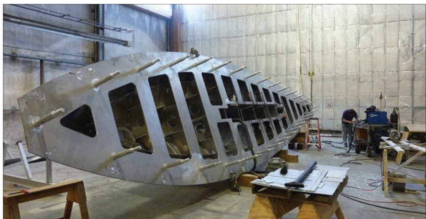
Left —Construction details of the forward sections of America 2.0. Note the marriage of the balsa-cored laminated-cedar hull skin to the aluminum ring frames and keel structure. Right —The welded aluminum lower section of America 2.0's hull and keel sump await attachment to the rest of the wood-and-aluminum hull. Note the massive threaded studs protruding from the flange that will secure the two structures to one another.
