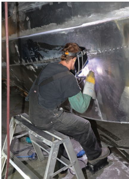
Welders work outside and inside the bow sections of the 60' (18.3m) Greg Marshall-designed whale-watcher catamaran.
